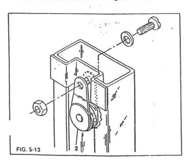
Install center pulley (2) in center channel with washer, bolt and nut. Finger tight. See Figure 5-13.
